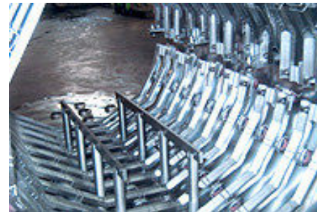
Wire Type and U Shape Mo Heating Elements (shown installed in a customer's furnace)
