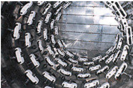
Wire Type and U Shape Mo Heating Elements (shown installed in a customer's furnace)
