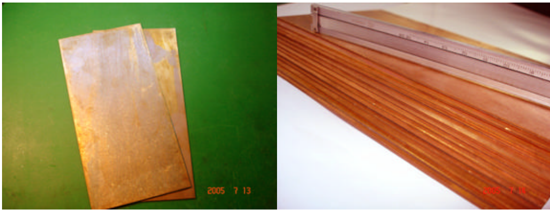
Fig. 6 Typical Cu/Mo70Cu/Cu Laminate Products
